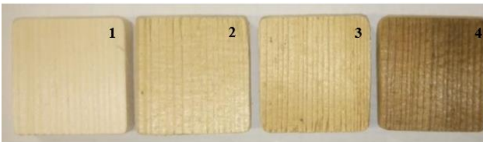
Fig. 1 Used samples. 1 – untreated control sample, 2, 3, 4 – heat treated spruce samples, at temperature levels: 2 – 160 °C, 3 – 80 °C, 4 – 200 °C
