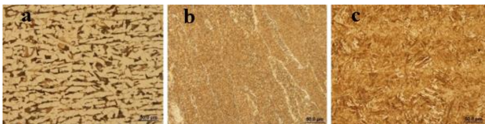
Fig. 5 Microstructure – light microscopy – input analysis of weldment a – basic material; b – weld joint; c – raking blade
