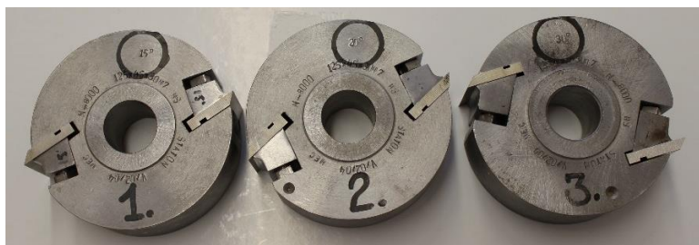
Fig. 3 Milling heads with rake angle of 15°, 20° and 30° Obr. 3 Frézovacie hlavy s uhlom čela 15°, 20° a 30°
