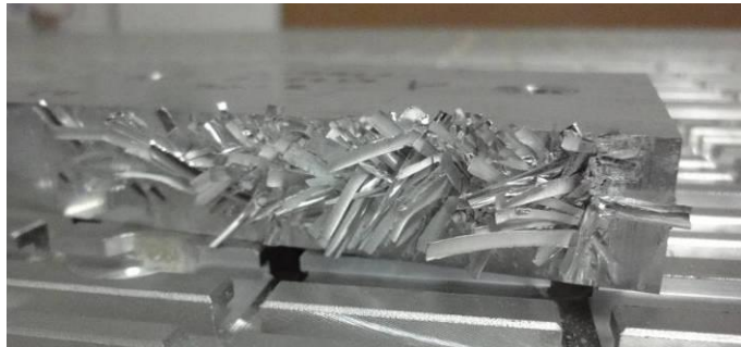
Figure 5 Chip welding on the workpiece
