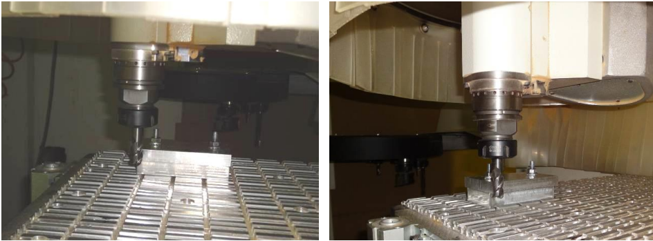
Figure 4 Specimen jigging and milling
