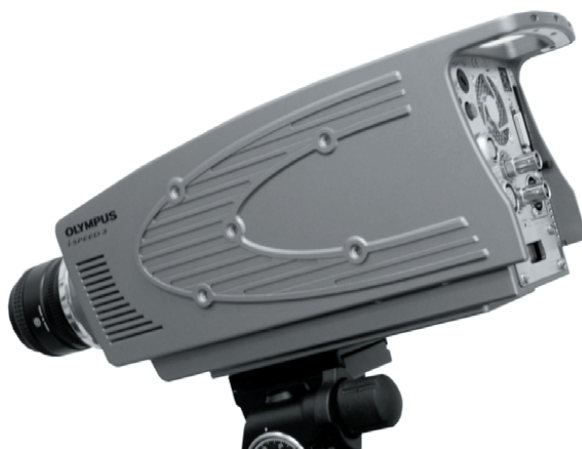
Figure 1 High-speed Camera Olympus i-speed 3
