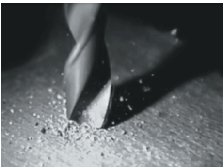
Fig. 11 Cast Iron Drilling, a) HSC Tip, b) SC Tip
