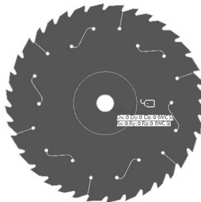
Figure 3 Model of circular saw blade clamped with function “constrain displacement”
