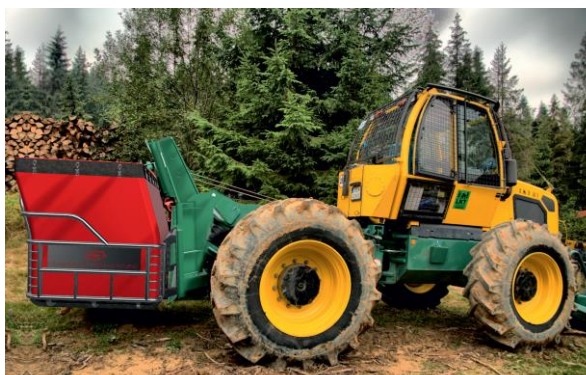
Fig. 3 The use of a base machine in fires in the forest, as a carrier of a detachable body
