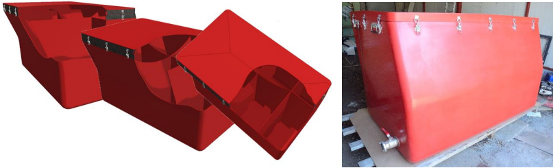
Fig. 4 The water tank construction with built-in wave-breaks
